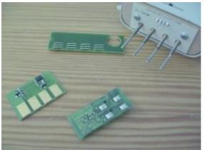
This instructions will try to help you using our resetter for laser toner chips found in Samsung (tm) toner cartridges. Device was designed to be as easy to handle and store as possible.
