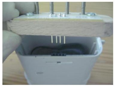
When connecting connector with resetter be carefull to place all 4 pins to resetter board located inside plastic housing.
