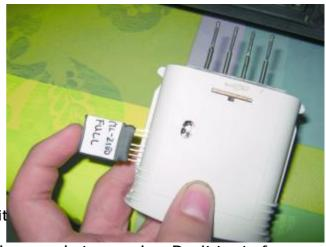
When inserting diskette be carefull that you insert it correctly. Diskette module has 6 pins which must
